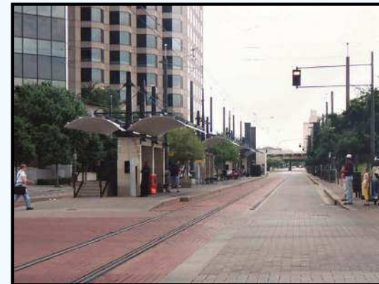
Multiple traffic lanes lost by LRT
