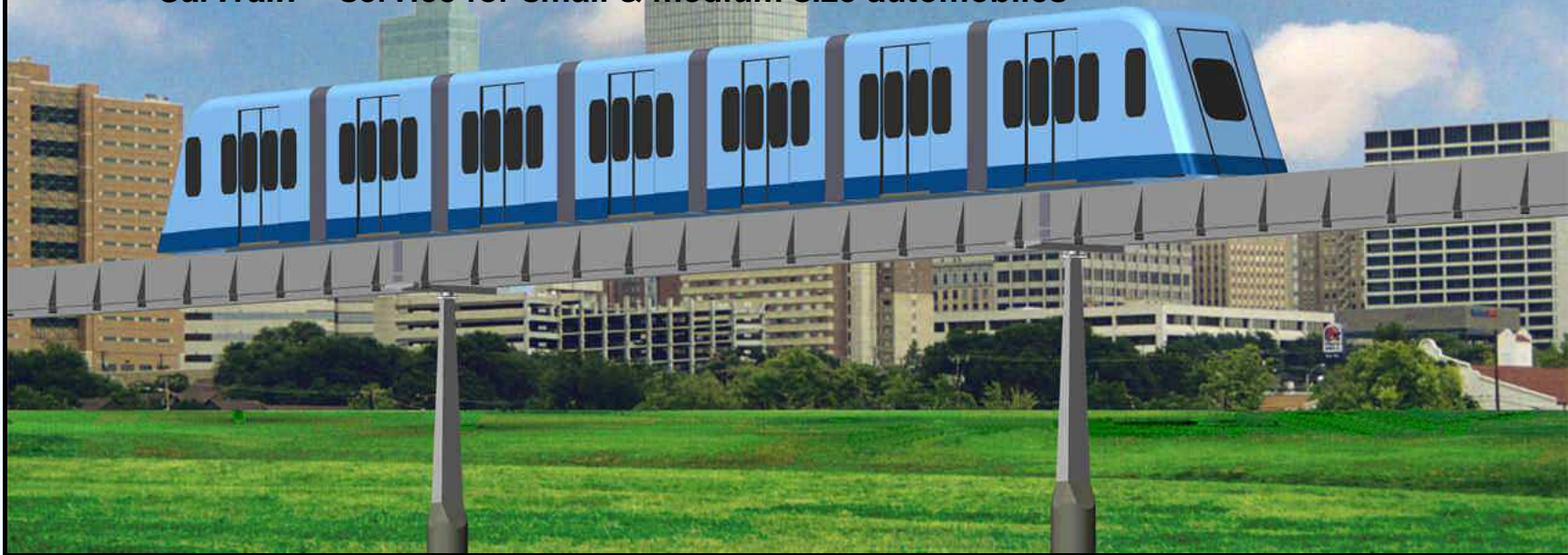
Ultralight MicroWay passenger transport train on elevated SuperWay ™ ( Mechanically-coupled train operated by on-board motorman )
