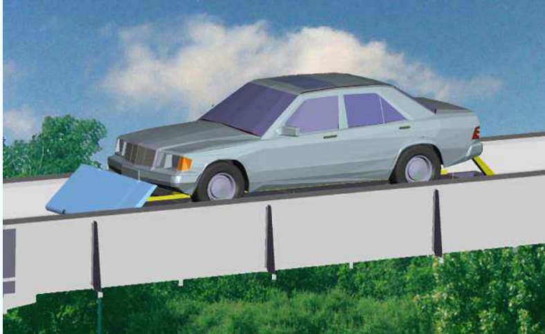
Carferries carry standard cars with driver and passengers inside
